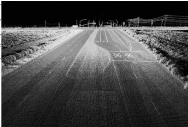
Mobile lidar can capture a large amount of data about road surfaces. New collection technologies provide more accurate information for transportation agencies
