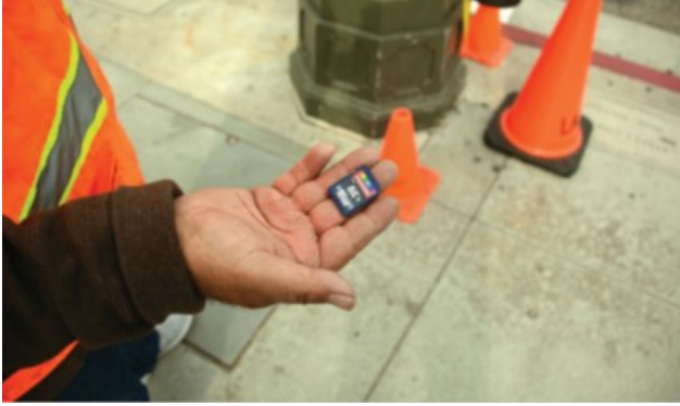
Video traffic count data is stored on a memory card. Storage and organization of large amounts of data is a concern for transportation agencies.
